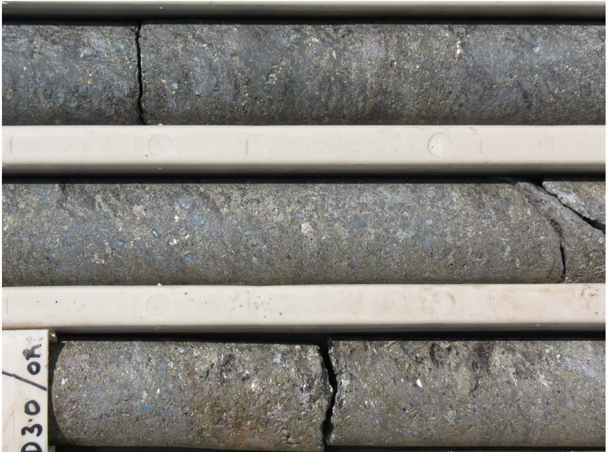
Photograph 2. One Mile Mining Lease – Close-up photograph of core from hole SPOM004 for part of the interval from 277.1m to 279.2m (Tray 14). The sulphides are mainly pyrite at the top and pyrite and chalcopyrite at the bottom.
