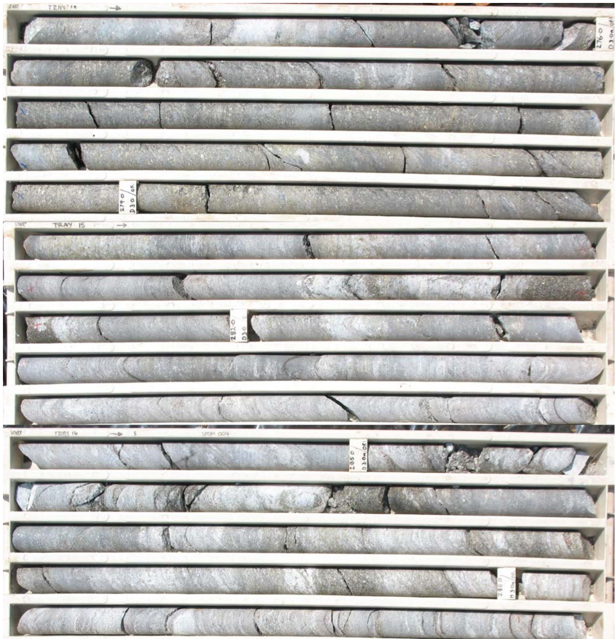
Photograph 1. One Mile Mining Lease – Photograph of core from hole SPOM004 for the interval 275m to 289m (Trays 14, 15 and 16). The sulphide content is significant throughout the interval with some semi-massive sulphides at the top and disseminated sulphides in strongly altered material at the bottom. The sulphides are largely pyrite but variable amounts of chalcopyrite and sphalerite occur in the top two trays.
