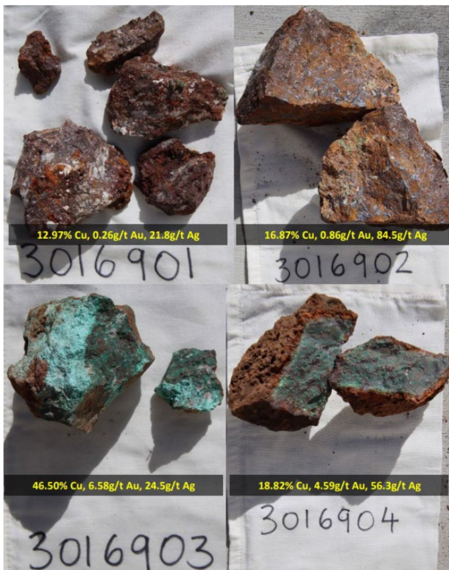
Figure 10. Mullock and rock chip samples collected from the Halls Reward Prospect. Sample 3016901 – copper oxide bearing ferruginous quartz, native copper and malachite; Sample 3016902 – copper oxide bearing ferruginous quartz, native copper, cuprite and malachite; Sample 3016903 – copper oxides chrysocolla and malachite; and sample 3016904 – copper oxide bearing ferruginous siliceous gossan, malachite needles, cuprite, spongy silica. 8
