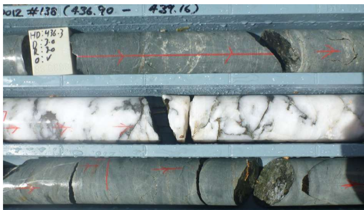
Figure 11. Core from BTDD012 (437.0 – 437.5m) with a 50 cm wide quartz-chalcopyrite-pyrrhotite-pyrite vein in strongly foliated and altered meta-andesite. The milky white quartz has been fractured and recrystallised with late sulphides infilling the fractures together with flakes of sericite. An intense quartz-sericite alteration selvage in andesite surrounds the vein.
