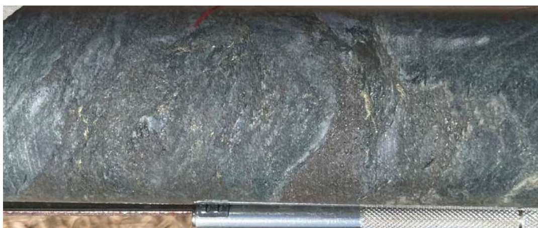
Figure 7. Core from BTDD011 (225.5m). Example of the two major types of hydrothermal alteration at Bottletree. Core sample consists of a moderately foliated meta-andesite with strong brown biotite (potassic) and later dark green actinolite (calcic) stages of alteration. Brassy yellow chalcopyrite is preferentially associated with biotite in this zone of “calcic-potassic” alteration. Alteration is preferentially focussed along pre-existing foliations.
