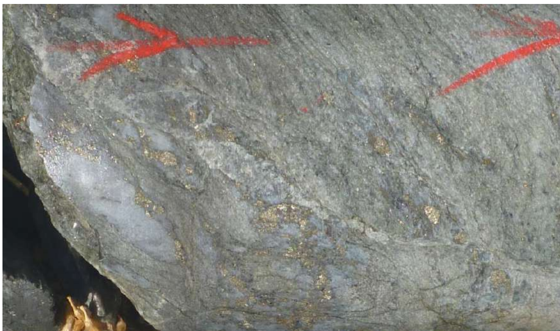
Figure 12. Core from BTDD012 (465.2 m). A sheared and fragmented 3 cm wide quartz vein consisting of 1-30 mm long fragments of grey quartz in an anastomosing matrix of sulphide minerals. Host rock is a strongly silicified and foliated quartz diorite.
