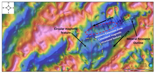
**Figure 12**. Aerial magnetic image (RTP) of the Cockie Creek regional area showing the outline of the historical Mineral Resource and the Western Extension Zone (red polygon) as supported by a linear series of magnetic features. A prominent large circular magnetic feature is located south of the Western Extension Zone (yellow circle).
