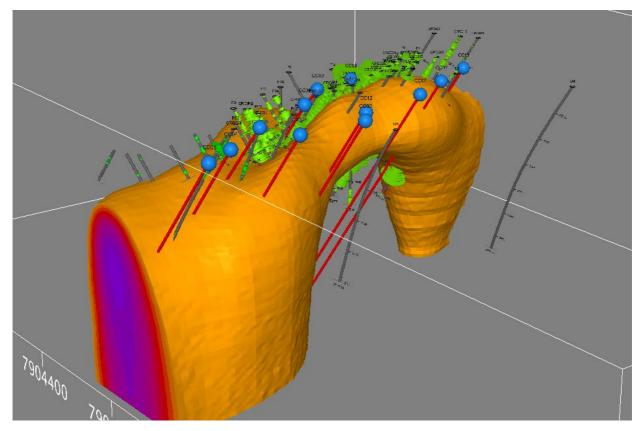
*Figure 13.* 3D IP chargeability model showing moderate to high chargeability zone. Historical drill holes (grey traces) and copper mineralisation (green) with 2023 planned drill holes in red. Viewed looking northeast.
