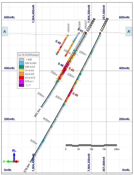
**Figure 3**. Cross-section (+/- 15m) taken along A-A' (as shown in Figure 2) looking east-northeast showing CCDD004 and CCDD006 plus historic CRC017 (twinned with CCDD004) and proximal historic drill holes CRC009 and CRC010. Down-hole copper assay values (1m intervals) are represented as grade categories.
