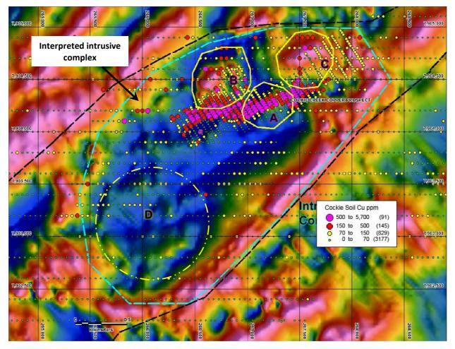
*Figure 15.* Cockie Creek thematic Cu soil data and interpreted porphyries on TDr VI NSSF processed airborne magnetics data, showing interpreted porphyry intrusions (A to D) within an interpreted intrusive complex.
