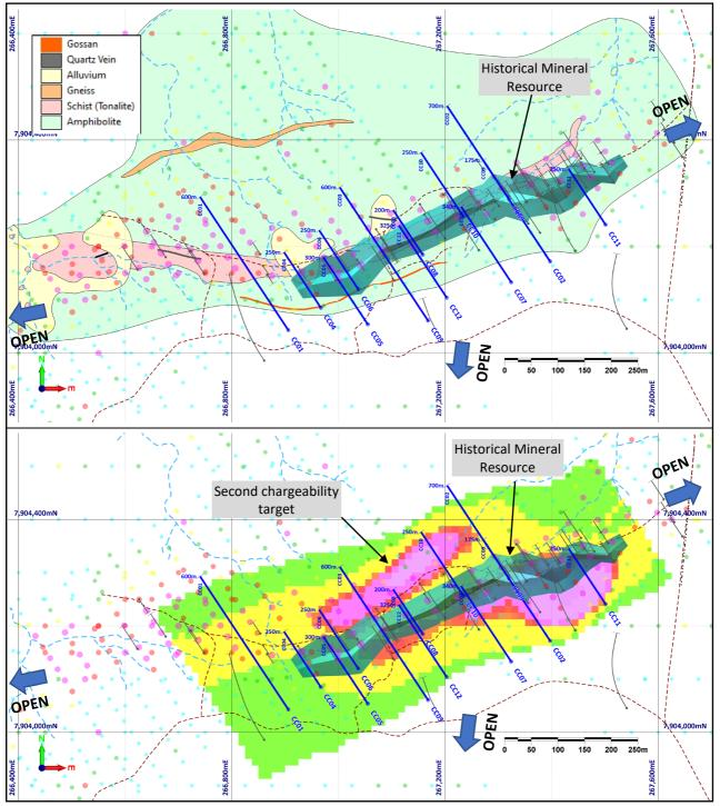
**Figure 14**. Plan views of Cockie Creek Prospect surface geology (top) and IP chargeability data (bottom). Gridded soil copper geochemistry, planned drill holes (blue traces) and wireframe of the historical Mineral Resource are shown in each plan.
