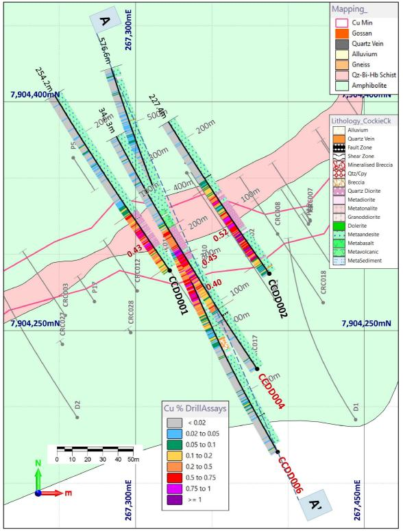
**Figure 4**. Plan geological map of the eastern part of the Cockie Creek deposit showing drill holes from the current program with new assay data (CCDD004 and CCDD006 labelled in red) and lithologies from core logging. Note that all drill holes have long intersections with good Cu grades in hanging wall meta-andesites above the Cu-Au mineralized zone in the intrusive rocks. Down-hole copper assay values (1m intervals) are represented as grade categories.
