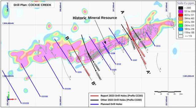
**Figure 2**. Plan map of the Cockie Creek Discovery Outcrop area showing completed drill holes (CCDD004, CCDD005, and CCDD006) with new assay data discussed in this release (in red), other 2023 drill holes reported in previous releases (in black), planned but not yet drilled holes (in blue) and historic drill holes (in grey) over gridded Cu soil geochemistry. Outline of historic Mineral Resource at surface and cross sections A-A' and B-B' are shown.
