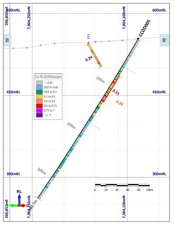
**Figure 5**. Cross-section (+/- 15m) taken along B-B' (as shown in Figure 2) looking east-northeast showing CCDD005 and proximal historic drill hole P25. Down-hole copper assay values (1m intervals) are represented as grade categories. The 0.20 label in orange indicates the lower grade interval of 120m @ 0.20 Cu% whereas the 0.31 label in red indicates the higher grade interval of 57m @ 0.31 Cu%.
