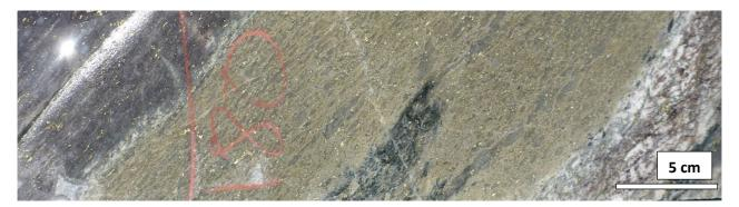
**Figure 8**. Core from CCDD004 (180 m) showing a 20 cm wide zone of intense greenish yellow sericite-chlorite alteration replacing pale brown potassic alteration (left contact) and greyish white albite and forest green actinolite sodic-calcic alteration (right contact). Note the disseminated brassy yellow pyrite and chalcopyrite in the foliations in diorite.
