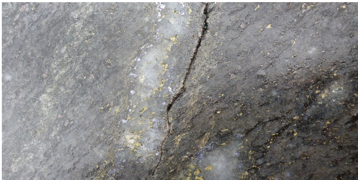
Figure 6. Core from CCDD003 (81.4 m) showing a typical recrystallized quartz-pyrite-chalcopyrite-molybdenite vein (1 cm wide) crosscutting foliation in a quartz diorite. Brassy yellow pyrite-chalcopyrite and steel grey molybdenite have been remobilized and redistributed to vein margins. Foliation is defined by the alignment of brown flakes of hydrothermal biotite (potassic alteration). Interval contains 0.66% Cu, 0.18 g/t Au, and 752 ppm Mo.
