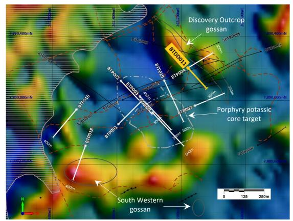
*Figure 5. Plan view of Bottletree Prospect area showing planned 2023 program holes (prefix BTP), current hole BTDD011 and 2021 and 2022 drill holes against aerial magnetic (RTP) processed image.*
