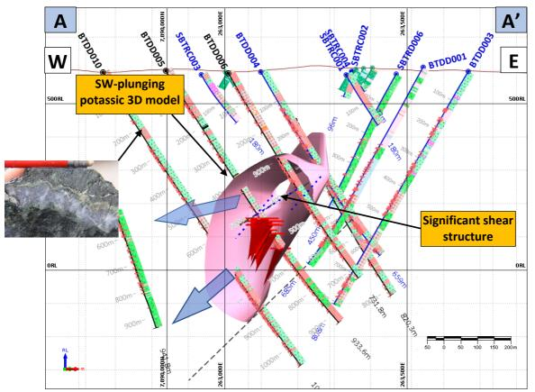
Figure 7. Cross section A-A' showing 3D model of the general zone of main potassic alteration which, based on alteration and structural information, plunges with a range of dips towards the south-southwest. Large blue arrows indicate possible vector directions towards a porphyry potassic core. An early-stage quartz-chalcopyrite vein is also shown.
