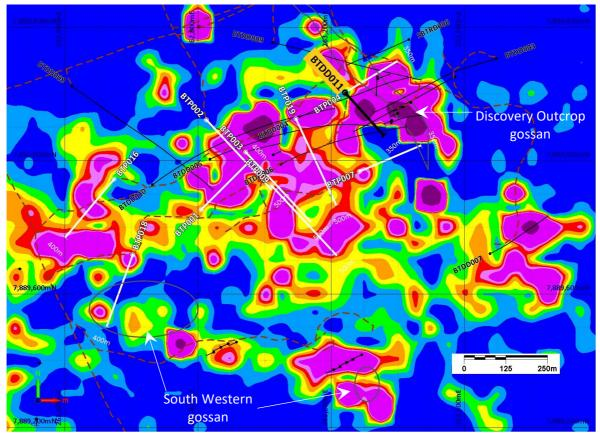
*Figure 3. Plan view of Bottletree Prospect area showing gridded Cu soil geochemistry, planned 2023 program holes (prefix BTP), current hole BTDD011 and 2021 and 2022 drill holes.*
