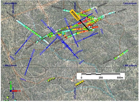
*Figure 2.* Satellite plan view of Bottletree Prospect area showing planned 2023 program holes (prefix BTP), current hole BTDD011 and 2021 and 2022 drill holes with Cu grade categories indicated as histograms along drill hole traces.
