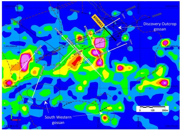
*Figure 4. Plan view of Bottletree Prospect area showing gridded Mo soil geochemistry, planned 2023 program holes (prefix BTP), current hole BTDD011 and 2021 and 2022 drill holes.*
