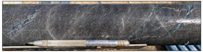
*Figure 9. Quartz diorite with chalcopyrite and pyrite mineralisation along foliation, with strong biotite and minor chlorite alteration (CCDD001, 64m).*
