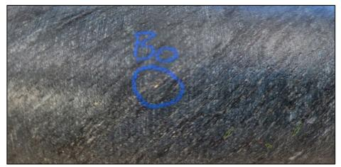
Figure 4. Diorite porphyry with disseminated chalcopyrite and bornite along strong foliation.
