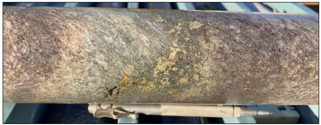
Figure 8. Quartz diorite with fracture-filled clusters of chalcopyrite and pyrite mineralisation (CCDD001, 50m).
