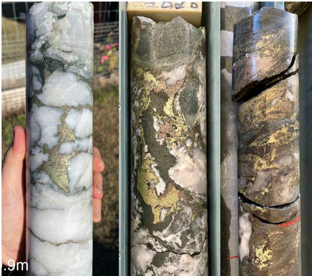
Figure 12. Examples of wall rock-hosted vein mineralisation: BTDD005 – 699.9m (left); BTDD005 – 708.5m (middle) – buck quartz vein with chalcopyrite-pyrite-pyrrhotite infill; and BTDD006 – 531.7m (right) – quartz-pyrite-chalcopyrite-pyrrhotite.
