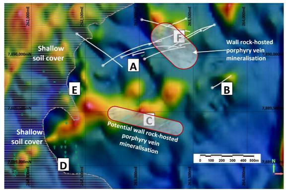
Figure 3. Plan of Bottletree diamond core drill holes over TDr Vi NSSF processed aerial magnetometer survey data. Porphyry Targets A to F with highlighted zones of more intense wall rock-hosted porphyry vein mineralisation and alteration zones are indicated.
