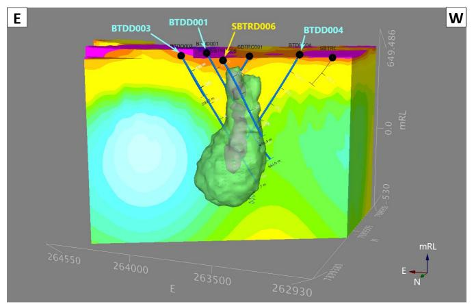
Figure 18. 3D-modelled MIMDAS IP high chargeability iso-surfaces representing the Bottletree IP chargeability anomaly, viewed looking southwest. Recently completed BTDD001, BTDD003, BTDD004 and 2018 drill hole SBTRD006 shown.
