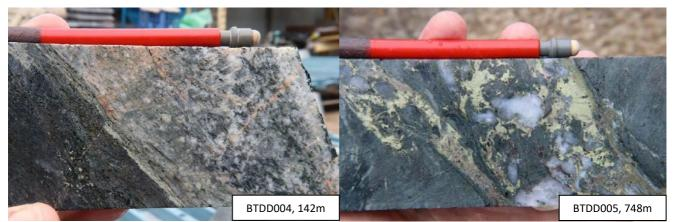
*Figure 5. Feldspar porphyry dyke (light coloured) with actinolite alteration intruded parallel to foliation (Left) and porphyry quartz-chalcopyrite-pyrrhotite D vein cross-cutting chlorite (photos from Corbett, 2023).*
