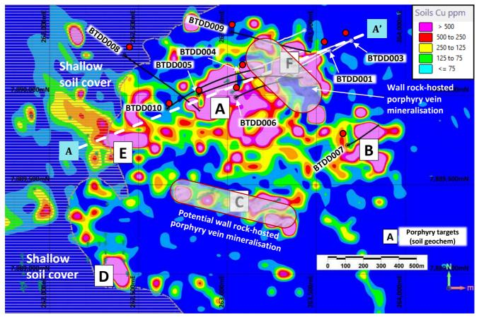
Figure 2. Plan of Bottletree diamond core drill holes over gridded soil copper geochemistry. Porphyry Targets A to F with highlighted zones of more intense wall rock-hosted porphyry vein mineralisation and alteration zones are indicated. Cross-section profiles in other figures are based on the dashed line A-A'. Area of recent alluvium and colluvium is shown as a hashed area over the western part of the image.
