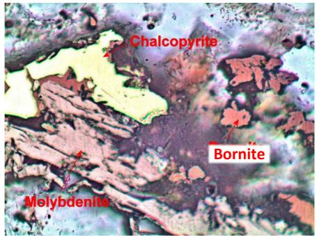
*Figure 14.* Thin section of highly altered dacite/tonalite porphyry (BTDD007, 95.30m) showing a chalcopyrite, bornite, molybdenite cluster. Reflected light. Width of frame: 200 microns (Taylor, 2022).
