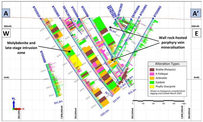
Figure 6. Down-hole intersections of porphyry alteration presented as key alteration minerals with histograms representing generalised alteration intensities. Modelling of the main potassic alteration fluid pathway (shown in 2-D), together with structural and other data, enables vectoring of the pathfinders towards a possible intrusion source for zoned alteration at depth to the west.
