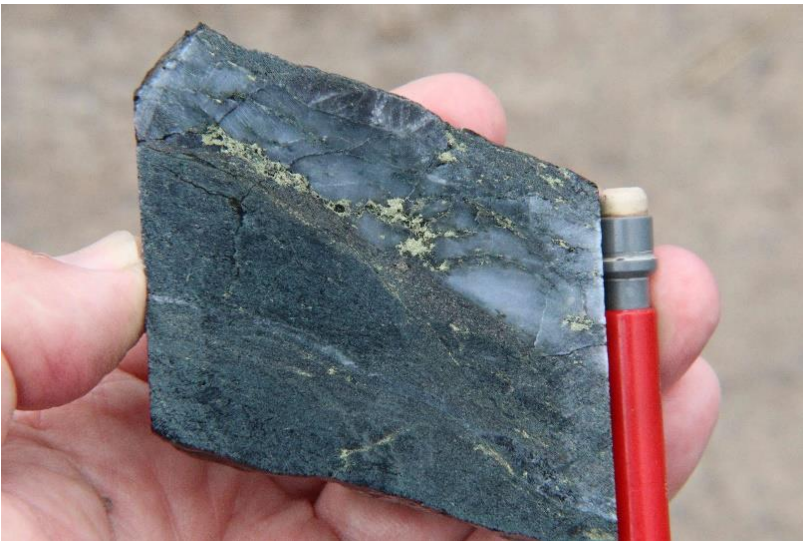
Photo 25 Quartz-chalcopyrite vein parallel to foliation in chlorite-actinolite schist, DDH BTDD005, 687.4m, 0.11% Cu.
