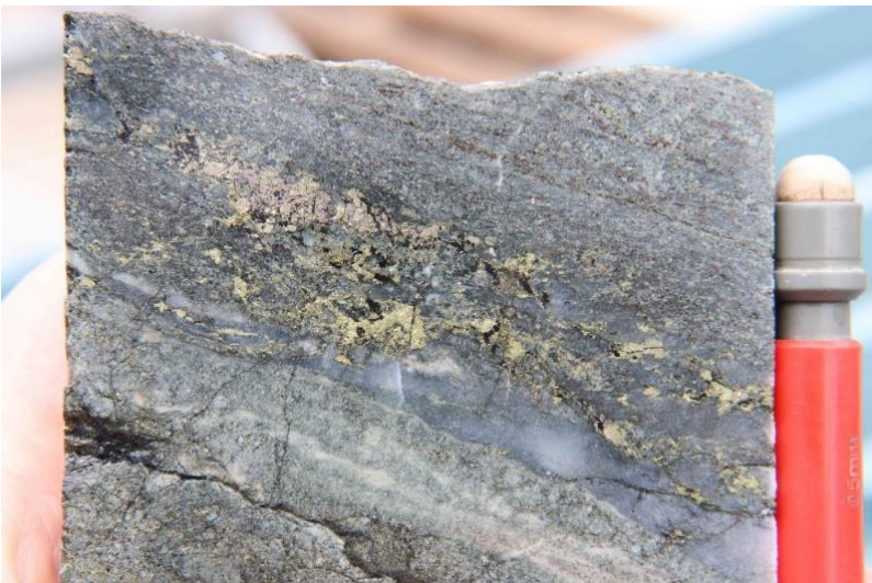
Photo 26 Quartz-pyrite-chalcopyrite vein with sericite overprint within the trend of foliation, DDH BTDD010 908.9m, 0.38% Cu.
