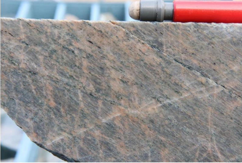
Photo 55 Foliated silica-chlorite-adularia alteration with sulphide in the foliation, DDH DTDD007, 318.7m.
