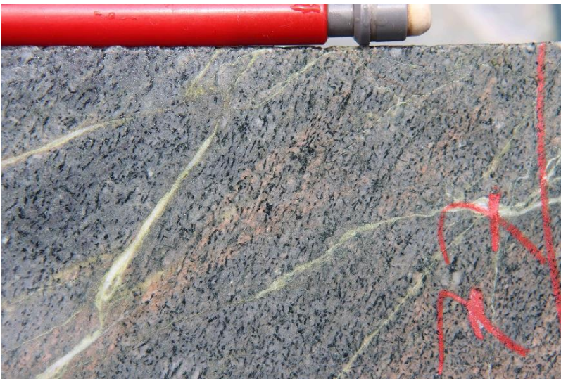
Photo 50 Actinolite partly aligned within the foliation with pink adularia, DDH BTDD010, 77m.
