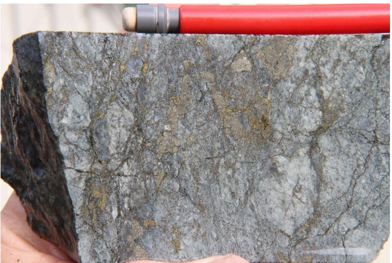
Photo 36 Pyrite-chalcopyrite mineralisation within sericite overprint within a fault with 0.12ppm Au and 0.6% Cu, similar to deep low sulphidation quartz-sulphide Au \pm Cu mineralisation, DDH BTDD4, 524.9m, 0.12ppm Au, 0.61% Cu, 3ppm Mo.
