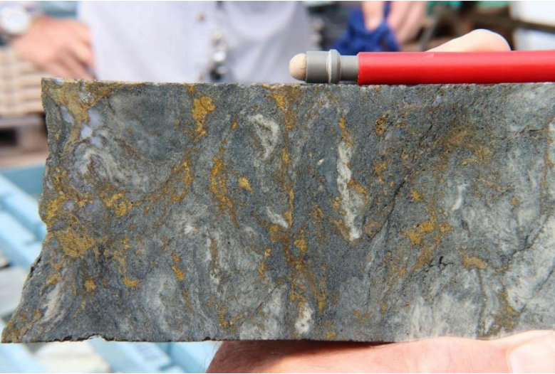
Photo 37 Chalcopyrite within complexly folded foliation in the footwall fault zone, DDH DTDD004, 632.3m 0.23ppm Au & 1.97% Cu, as part of 6m @ 0.8% Cu.
