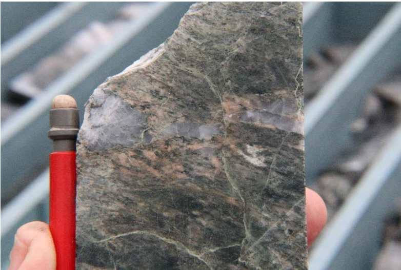
Photo 53 Silica-chlorite alteration with foliation-parallel quartz veins with Kfeldspar (adularia or orthoclase) selvages, DDH BTDD005, 639.4m.
