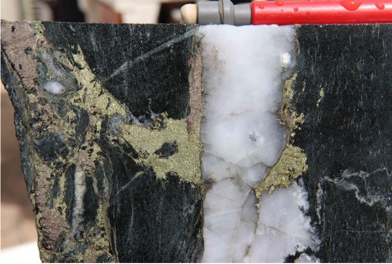
Photo 24 Quartz-pyrite-pyrrhotite vein initiated within foliation but also cutting it DDH BTDD005, 727.1m, 0.71% Cu.
