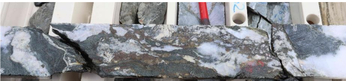
Photo 33 Mineralised quartz-sulphide vein parallel to the core axis that terminates at two cross structures in a sigmoid shape, DDH SBTRD006, 361.5m, 0.63%.
