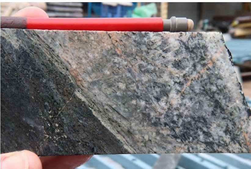
Photo 23 Feldspar porphyry dyke with actinolite alteration emplaced parallel to foliation, DDH BTDD004, 142m.
