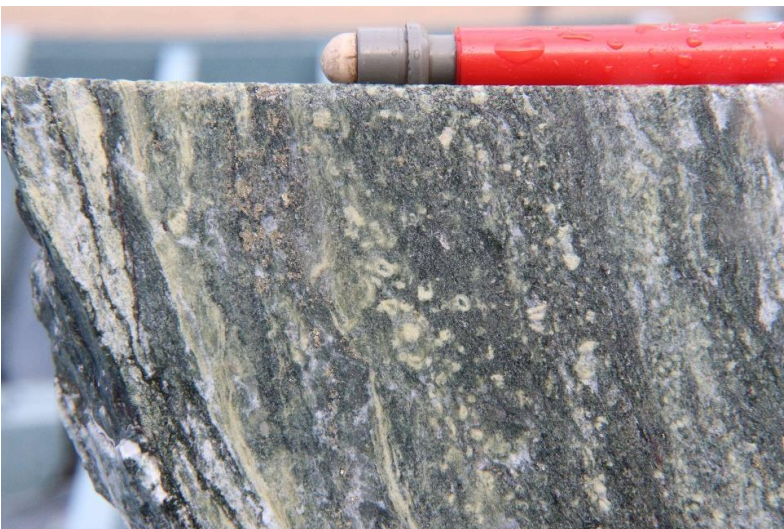
Photo 60 Shear with quartz-chlorite-carbonate-epidote-pyrite-chalcopyrite, DDH BTDD007, 268.7m, 835ppm
