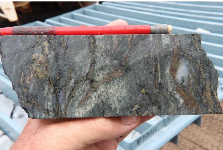
Photo 47 Strongly foliated rock with pyrrhotite (LHS) and a D vein with pyrite-chalcopyrite possible bornite (RHS) and minor secondary biotite with sericite overprint, DDH BTDD010, 1022.8m, 0.19% Cu & 2.7ppm Mo.
