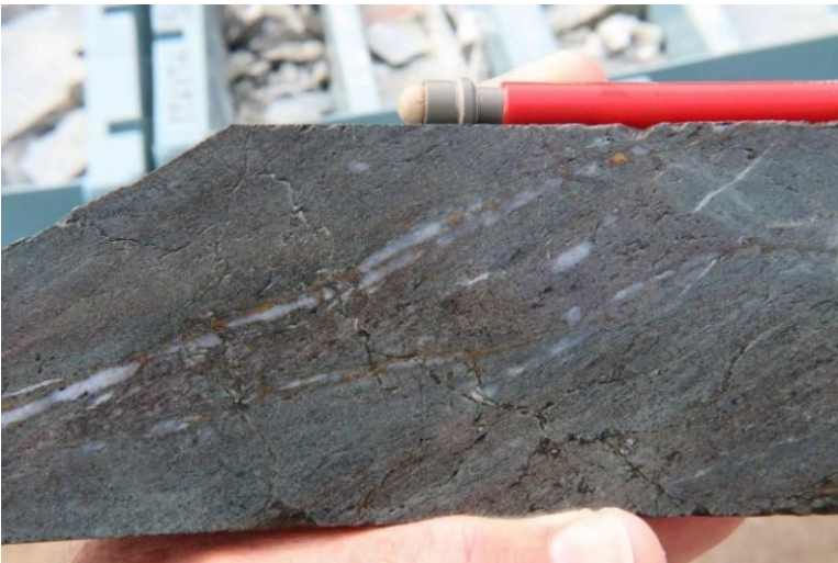
Photo31 Quartz-biotite-chalcopyrite shear parallel to foliation, DDH BTDD004, 281.9m, 0.17% Cu.
