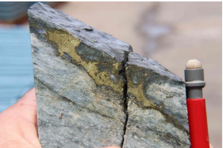
Photo 39 Quartz-chalcopyrite exploits foliation near fault 0.1ppm BTDD004, 637.3m, 0.1ppm Au & 0.48% Cu, as part of 6m @ 0.8% Cu.
