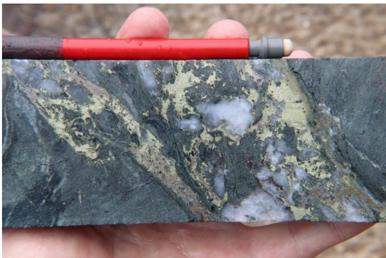
Photo 43 D vein characterised by quartz-chalcopyrite-pyrrhotite and yellow-red sphalerite cross-cuts and folds chlorite, BTDD005, 748.3m, 0.12% Cu, 1.2ppm Mo.
