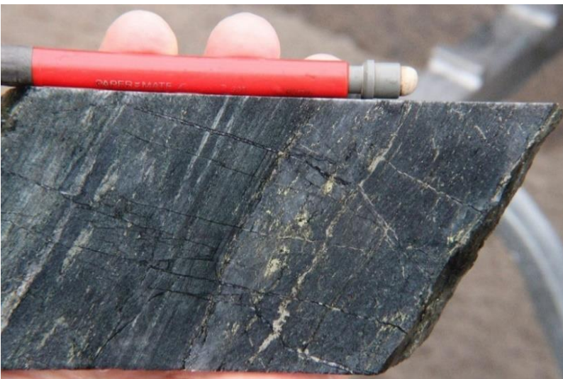
Photo 8 Strongly developed foliation with partings exploited by sulphides, some compositional layering and a ghosted fold on the left, DDH BTDD005. 661.3m. 3363ppm Cu.
