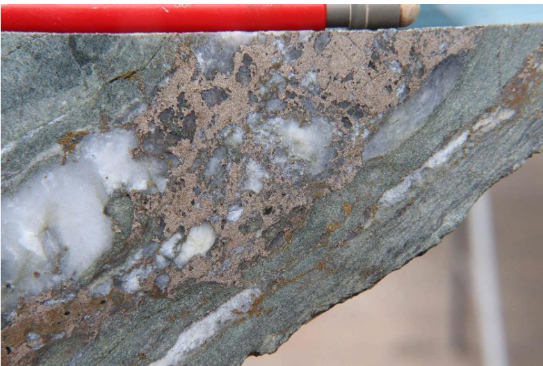
Photo 35, Quartz-chalcopyrite-pyrrhotite vein aligned within the foliation at a modest angle to the core axis, DDH BT004, 598.1m, 0.13% Cu.
