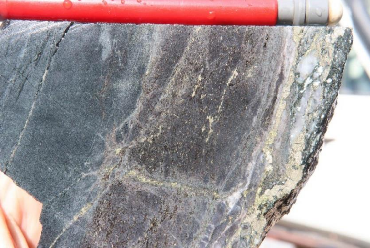
Photo 30 Foliation parallel zone of biotite-pyrite-chalcopyrite alteration within chlorite, and with a later D vein at the RH margin, DDH BTDD010, 898.1m, 0.27% Cu.
