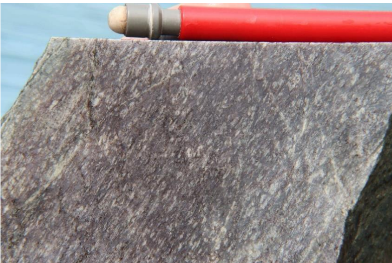
Photo 5 Penetrative foliation developed in a tonalite with biotite and lesser epidote alteration, DDH BTDD004 625.7m.
